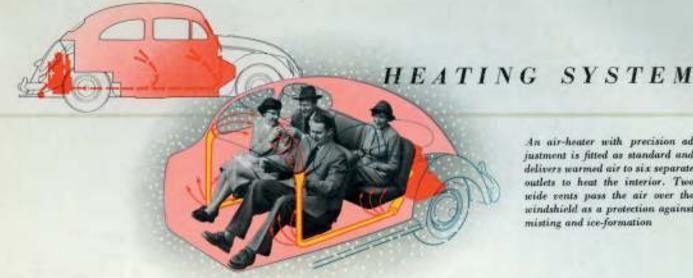
An air-heater with precision adjustment is fitted as standard and delivers warmed air to six separate outlets to heat the interior. Two wide vents pass the air over the windshield as a protection against misting and ice-formation
