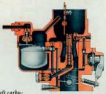
A special Solex downdraft earburettor of the latest type embodying an accelerating pump is fitted and gives the engine excellent response, brisk acceleration, lose consumption and a high degree of flexibility. Even at very low temperatures the engine starts easily; for progressive raising of the idling speed, the starter air valve is interconnected with the throttle
