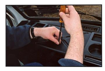
3. Using the screws provided, screw the tidy to the dash, ensuring you do not screw down too hard as this will damage the tidy.
