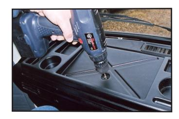
2. Position your tidy onto the dash top. When you are happy it is sitting correctly, drill pilot holes through the tidy and into the dash top at the points in the middle of the large flat area and the 'pen holder' on the left hand side of the tidy.
