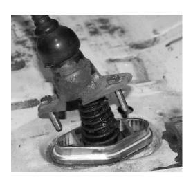
5. With the vehicle in second gear the base of the gearstick should be at 90° to the floor. If it isn't you need to move the base forward or backwards until the gear stick is at a right angle to the floor. Once this is achieved, tighten the bolts and replace the floor mat.
