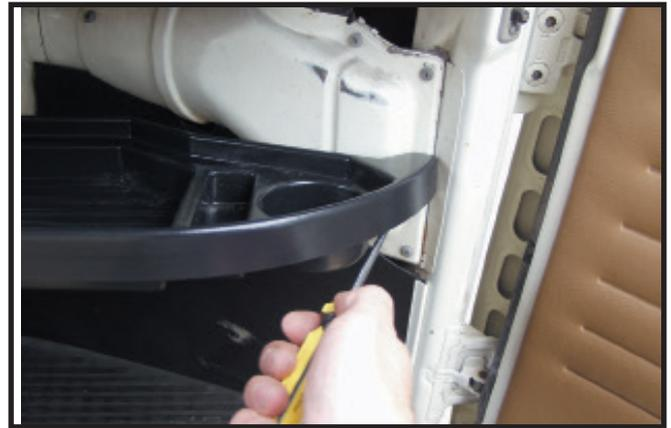
12. To attach the rear of the tray, hold the tray level using a 4mm drill bit, drill through the hole made previously, into the front bulkhead. Then screw the tray in place.
