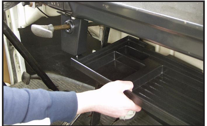
10. Hold the other end of the tray level, and using a 4mm drill bit, drill a hole through the tray into the front pillar.
