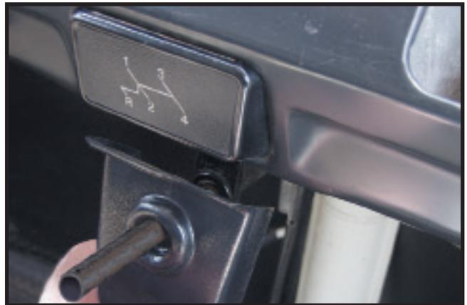
8. Screw the central mount to the dash using the large screws removed earlier and replace the handbrake handle.
