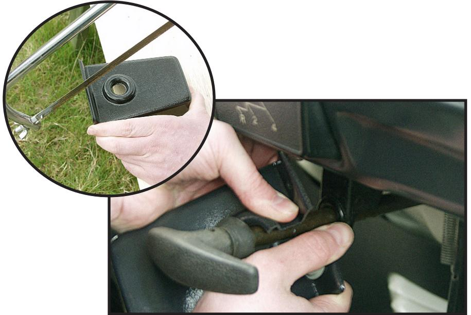
9. Offer up one of the under dash trays and bolt it into place using 1 nut, 1 bolt and 2 washers.
