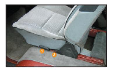
2. Once the seat is removed, you will see a plastic insert on one of the runners. This will need to be removed and put to one side.
