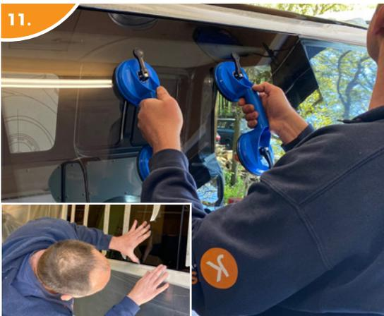
Before you lift the glass up, put 2x 400mm lengths of 50mm wide masking tape loosely along the roof edge,
