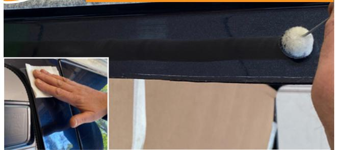
Clean the panel work with the alcohol wipes. Now apply the primer in a line, remembering the same will be done on the glass and between the two lines of primer will sit the bonding mastic.
