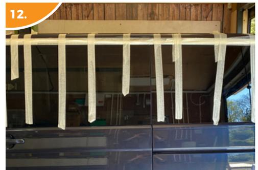
Once you are happy with the glass positioning and it's all taped up, remove protective masking (but not tape holding the glass in place), vacuum out the metal / dust in the rear of the vehicle and have a cup of tea.
