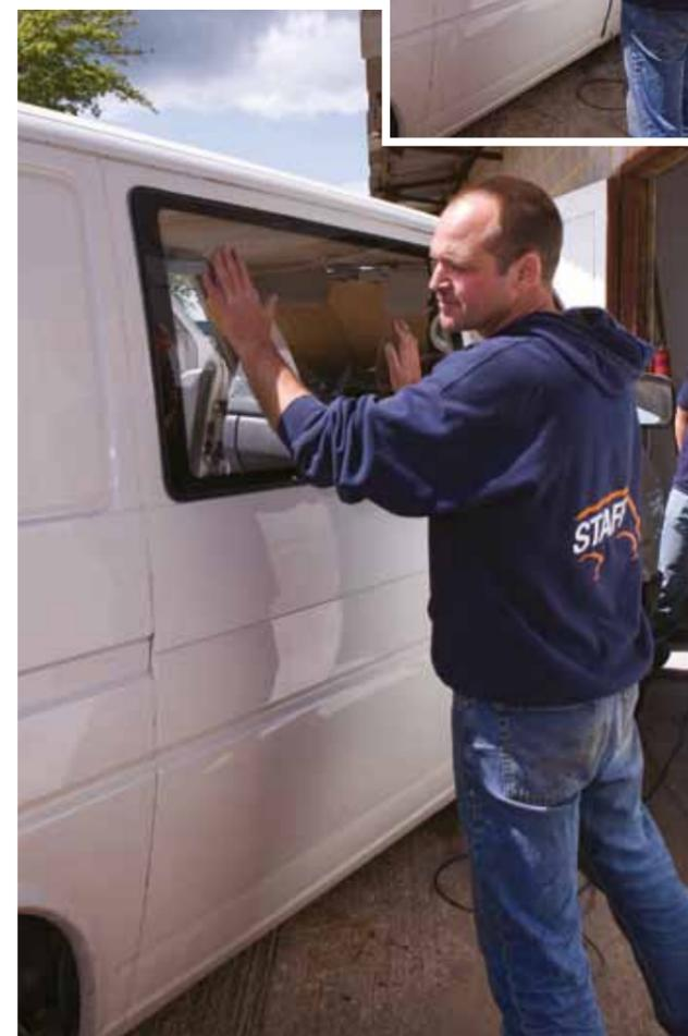
**13 SEALANT** With the correct piece of glass for the side of the Van you're working on laid out on a bench or similar, run a thick bead of adhesive all the way around the edge. A piece of card or dust sheet to protect the face of the glass is a sensible move here
