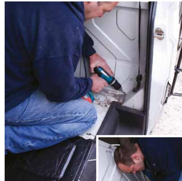
**04 DRILL** With the interior stripped out, it's time to break out the power tools. Type 2s are simple creatures so you can easily see where they're spot welded together. Work your way along the bulkhead and drill out all of the spot welds. Having a couple of spare drill bits on hand is a good idea as breakages can slow you down. You can use a centre punch on the spot welds to guide a normal drill bit, but it's easier and quicker to buy a proper spot weld drill bit
