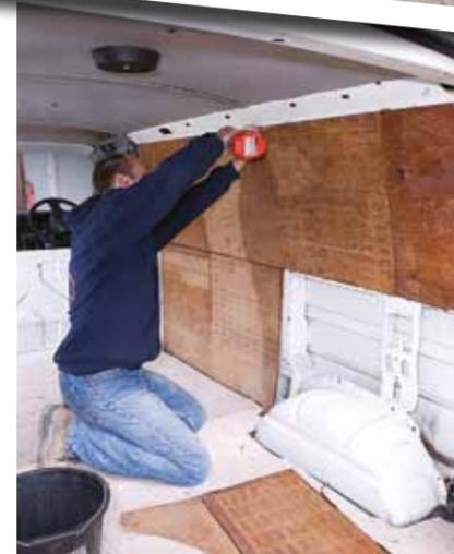
**02 THE STRIP DOWN** Our Van had been ply lined, which was a real bonus as it had prevented the Bus' metal sides from being damaged by stuff flying around inside. An electric drill took the effort out of this job
