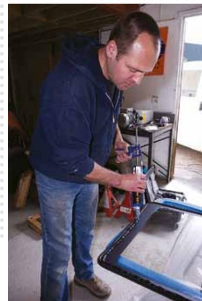
**14 FIT IT UP** Be careful how you hold the pane of glass (window suckers are a great idea) as you don't want to drop it or smere the sealant all over the place. Line it up and push it into position in one fluid movement as the adhesive will grip straight away. You can move it slightly if needs be, but don't try and lift it out again or you'll trap air in the glue and that will weaken the join
