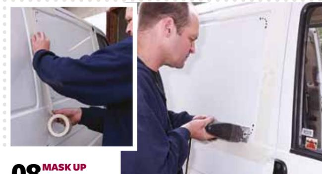
**08 MASK UP** ...move outside now and you'll see your pilot holes in the corners of the panel to be removed. Run some masking tape to protect the paintwork and then grab your jigsaw. You can make life a little easier for your jigsaw blade by enlarging the holes with a fatter drill bit but it isn't strictly necessary. Now simply join the dots, but take it easy and let the blade do the work
