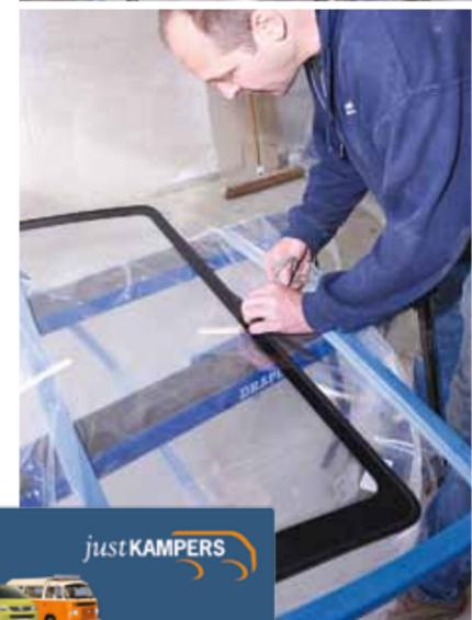
**12 TRIM TIME** The Just Kampers window kit comes with a piece of rubber finishing trim that runs around the edge of the glass. Fit this on the outer edge and cut off the excess with a knife or a sharp pair of scissors
