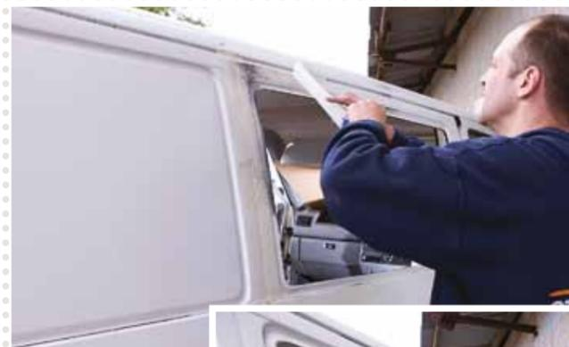
**11 PANEL PREP** The adhesive / sealant should do a good job of protecting the metal but it makes sense to paint the exposed metalwork. Allow it to dry and then give the paint a key to help the glue adhere to it. We had a piece of 40 grit sandpaper to hand so that's what we used
