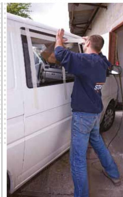
**15 TAPE IT UP** Use plenty of masking tape to hold the new window in place. You can't drive the vehicle for at least 24 hours whilst the adhesive sets. It goes without saying that it's a good idea to have somewhere out of the elements to store the Bus for this period of time
